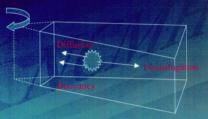
Centrifugation + Buoyancy + Diffusion =0 therefore particle acquires a velocity through the solution just enough to make the overall force zero
