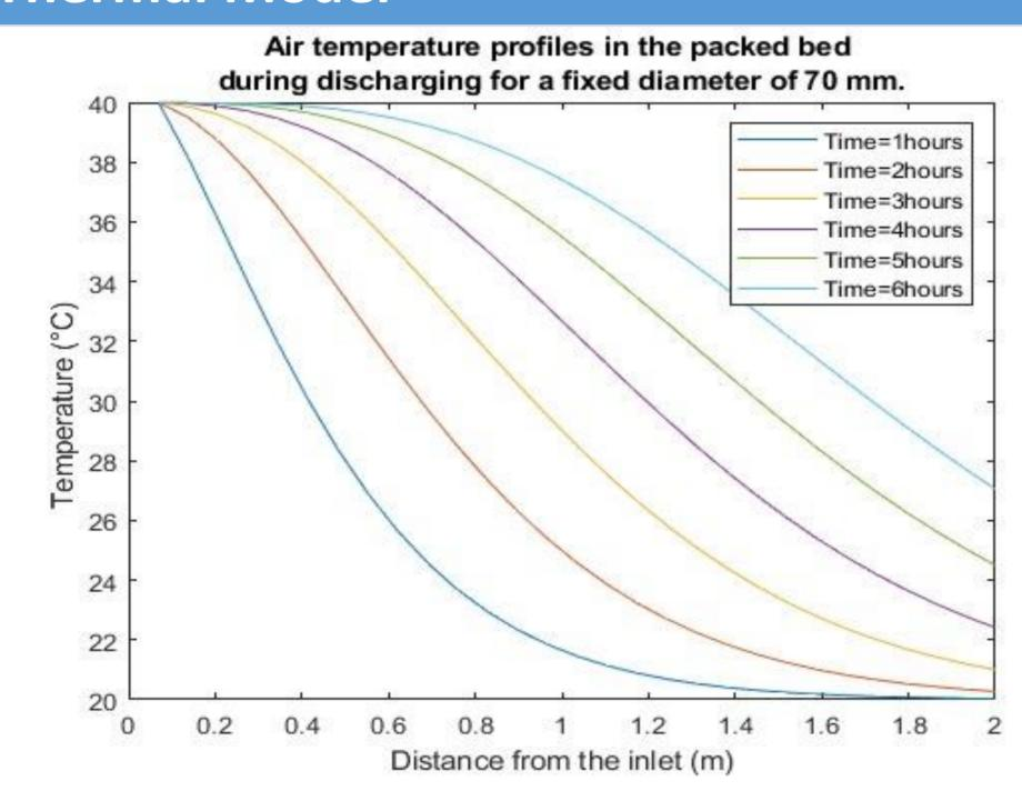
Cold energy will be stored during the night within the rocks in a packed bed and released during the day to cool down condenser. A fan will be used during days and nights to force air into the system. It is very important to be able to properly predict the temperature profile within the packed bed since it enables to optimize the charging time during the night and the outlet temperature of cooled air during operations. Thus, it enables us to evaluate energy savings.
