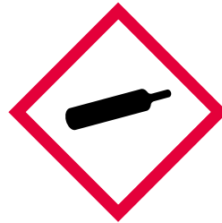
Gas under pressure
