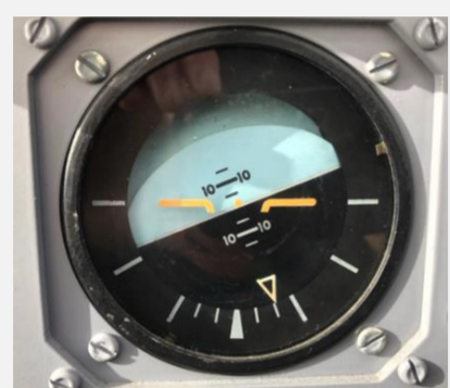
Figure 1. A Typical Attitude Indicator
