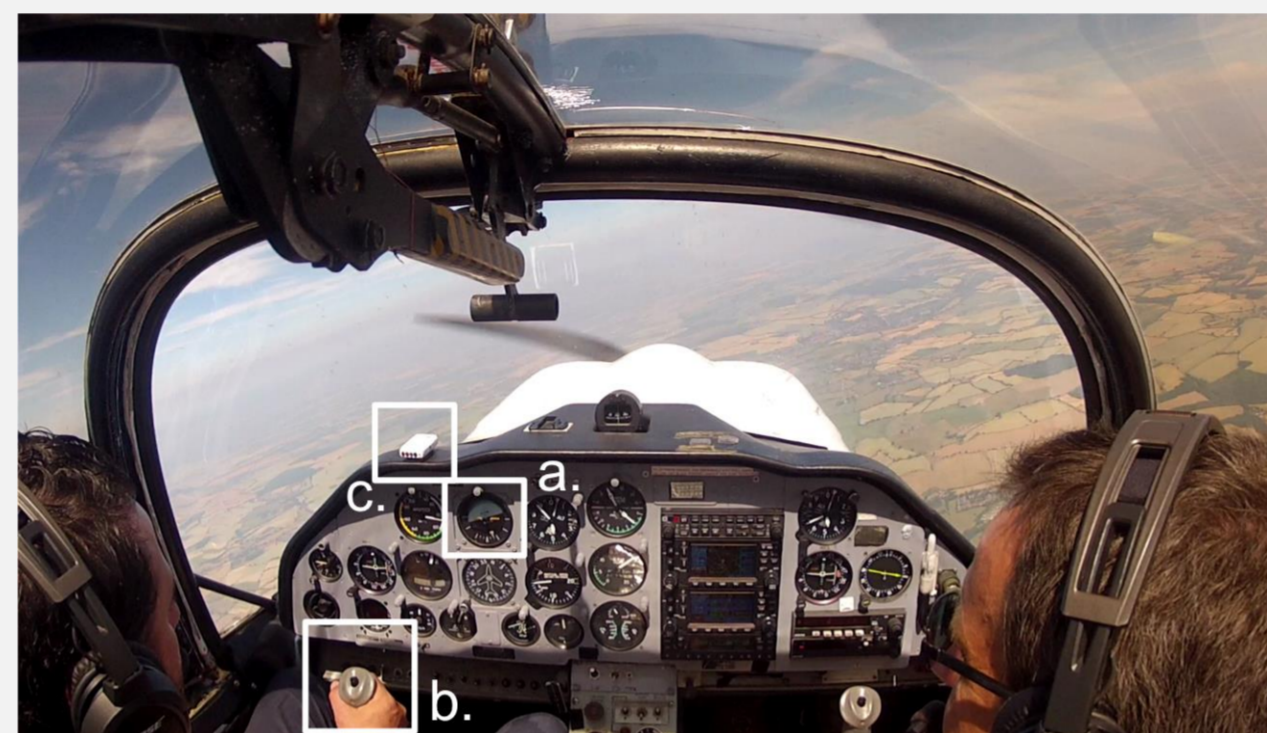
Figure 3. A screenshot of the cockpit video, showing (a) the AI, (b) the subject holding the centre-stick, and (c) the inertial measurement unit.
