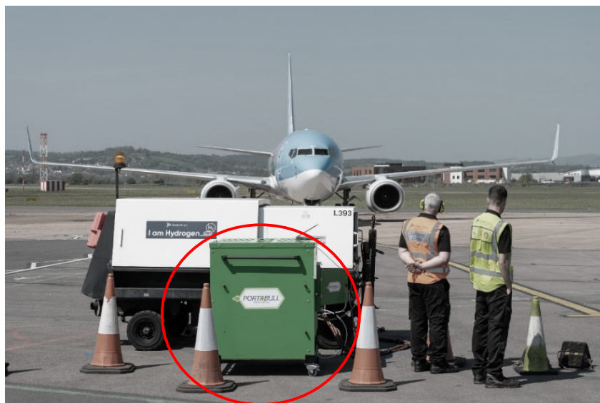
Figure 3 HyGPU with Portabull (circled) configuration during Zero Carbon Turn trial, April 2025
