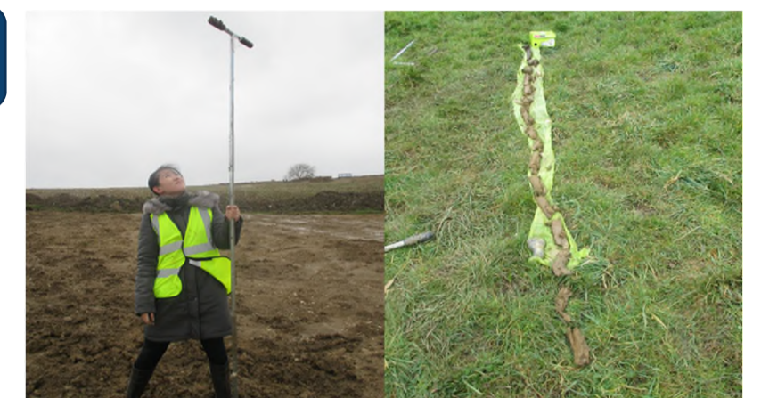
Images showing on-site soil sampling activities; (left) soil sample augering; (right) collecting soil samples for different augered depths
