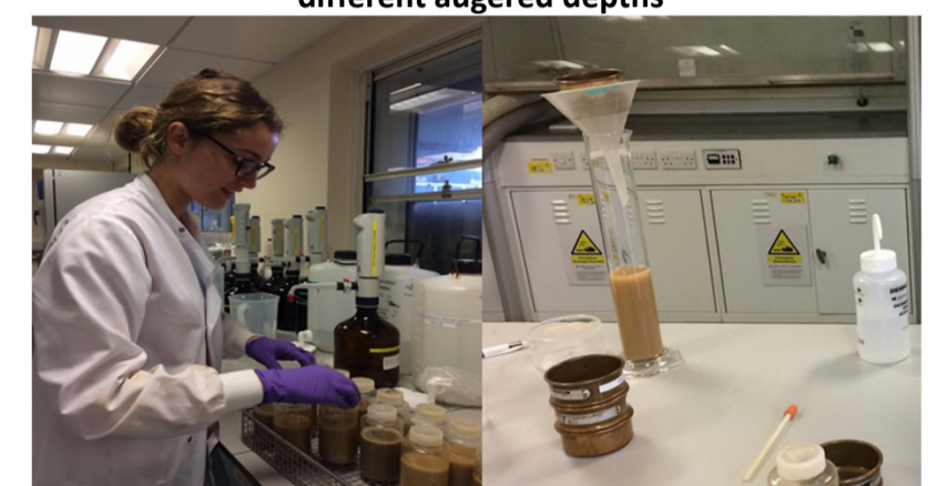
Particle size distribution analyses using sedimentation and pipette method in the laboratory
