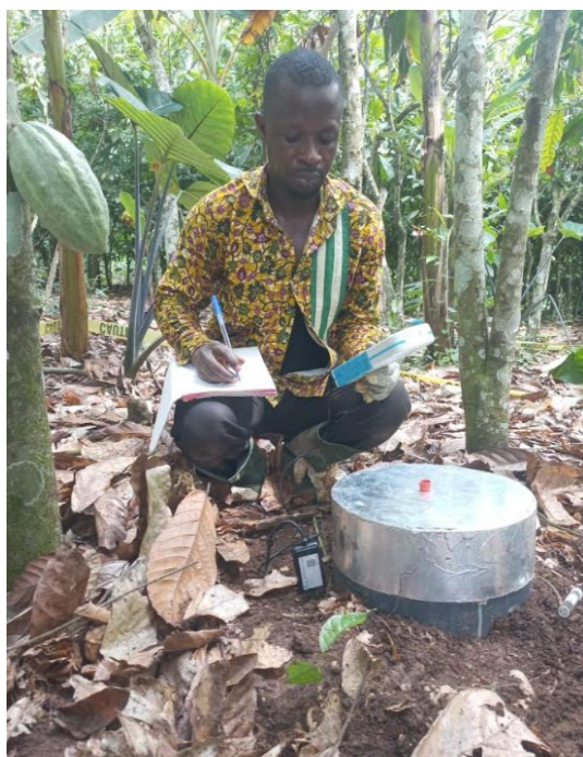
Soil moisture & temperature reading during GHG sampling
