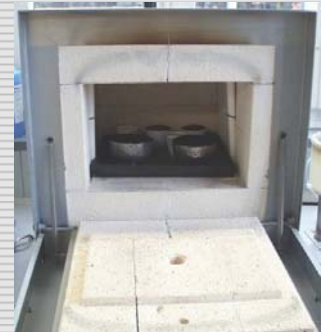
Ashing / calcination in muffle furnace at 600°C – 800°C
