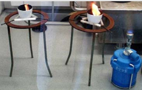
Ignition / burning of NC saturated with liquid paraffin
