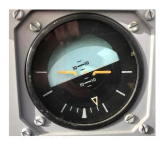
Figure 1. An example of a moving-horizon type AI, as used in this study, displaying a bank to the right.
