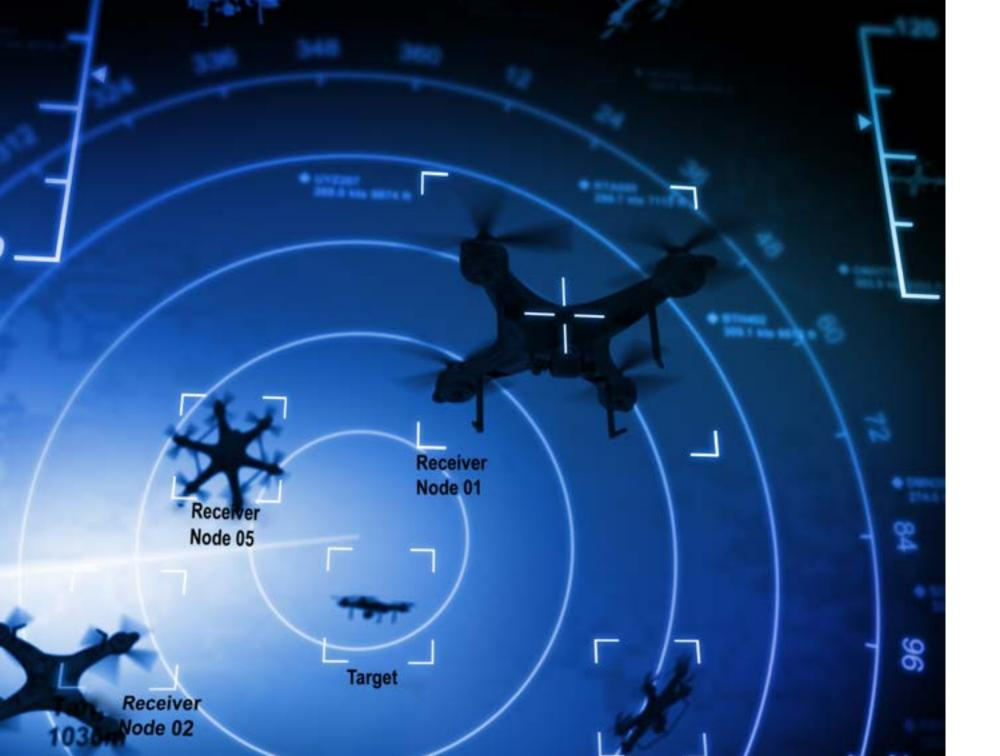
Development of a co-operative multistatic radar network based on the Aveillant holographic radar Staring radars use a transmitting static wide-beam antenna and a directive digital array to form multiple simultaneous beams on receive. Because the beams are static, the radar can employ long integration times that facilitate the detection of slow and low-reflectivity targets, such as drones, which present a challenge to traditional air surveillance radar.
